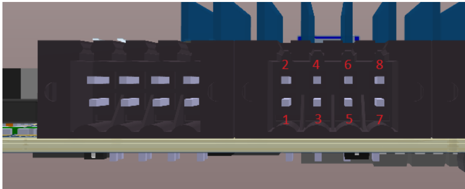
Figure 7: Pinout of J14 connector for RS-232 and RS-485 interfaces.
